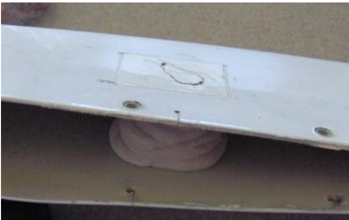
Excess bondo in a wingtip fairing—instead of making a proper repair
